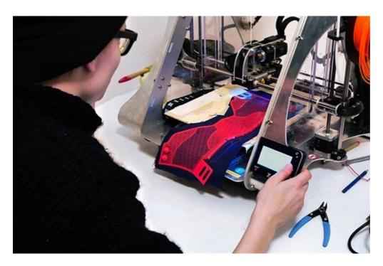
Constructed from flexible, biodegradable filament and natural textiles, the sneaker prototype is made using a ZMorph multitool 3D printer. While the duo initially struggled to find a way to stiffen the shoe's upper, it was a battle that unearthed an astonishing lesson: by printing the filament directly onto the material, Gronowicz and Motylinska found they were able to construct the entire shoe without using glue, making it more even more environmentally friendly and durable.
