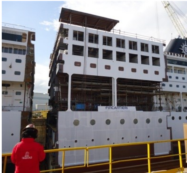
MSC Sinfonia, currently at the Fincantieri's shipyard in Sicily undergoing stretching as part of the Renaissance programme
