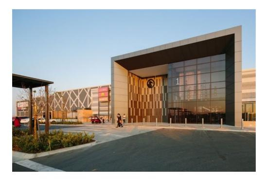
Unique dog leg entrances were designed at Springs Mall to create a wind break removing the need for expensive revolving doors. "It was a challenge to create the axes of the entrances in such a way that the wind can't get around the dog legs, but we are happy with the outcome."
