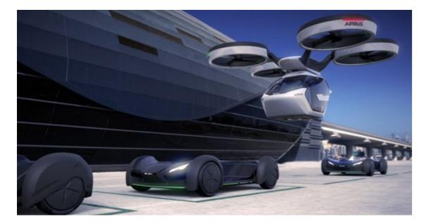
For megacity journeys, the capsule disconnects from the ground module and is carried by a 5m x 4.4m air module propelled by eight counter-rotating rotors. In this configuration, Pop.Up becomes a self-piloted air vehicle, taking advantage of the third dimension to get from A to B while avoiding traffic congestion on the ground.
