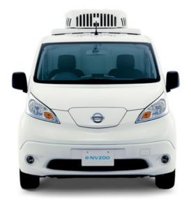
The ambulance also carries a lithium-ion auxiliary battery that supports life-saving medical equipment when patients are in remote areas or in need of emergency assistance. It also contributes to CO2 reduction, as well as external and internal noise reduction.
