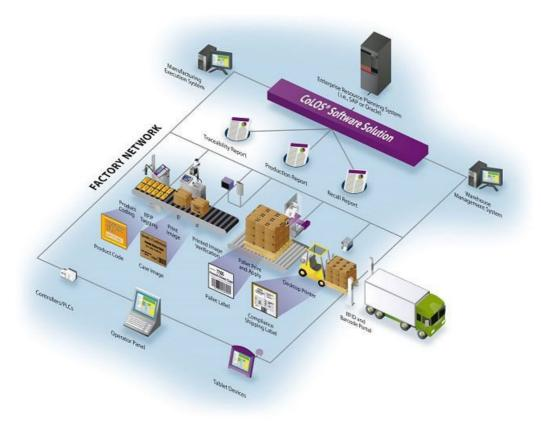
Confirming that products are properly coded while on the production line – at the precise time they are printed – CoLOS® Mark & Read minimises scrapped production and factory rework while preventing recalls. However, the level and type of verification required varies greatly. To better address this array of needs, Markem-Imaje, represented in South Africa by Pyrotec PackMark, has integrated three additional cameras within its 'Mark & Read' code verification portfolio.
