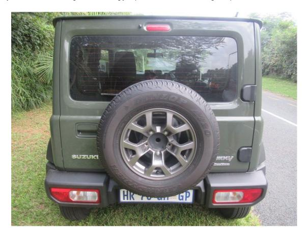
At the rear of the vehicle, Suzuki designers have moved all the lights into the horizontal rear bumper, which has allowed them to create a wider rear door, for increased practicality.
