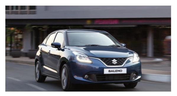
**Baleno GLX**: The GLX specification grade offers everything on the GL list, but with some additions and upgrades. Viewed front on, the headlights represent the most noticeable difference. They feature HID projector elements and LED daytime running lights, while low-mounted recessed fog lamps are standard, too. The exterior mirror housings incorporate integrate turn indicator repeaters.
