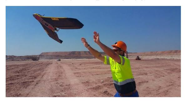
"Routine tasks historically carried out by surveyors, such as measuring the volume of waste dumps and stockpiles, are now being done by our drones. They collect digital imagery that is pieced together to perform volume calculations, giving us reliable data without having put anyone at risk," says Bongi Ntsoelengoe, technology manager at Kumba Iron Ore.
