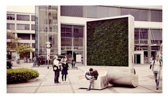
The green wall takes up  $3.5\text{m}^2$  in floor space and is just under 4m in height. It includes a sleek bench seat on both sides, as CityTree is designed to be situated in open public spaces, and room for poster advertisements on its flanks. It is a supercharged version of a natural crop of woods, emitting oxygen while scrubbing the local air of dust, nitrogen dioxide and ozone gases.
