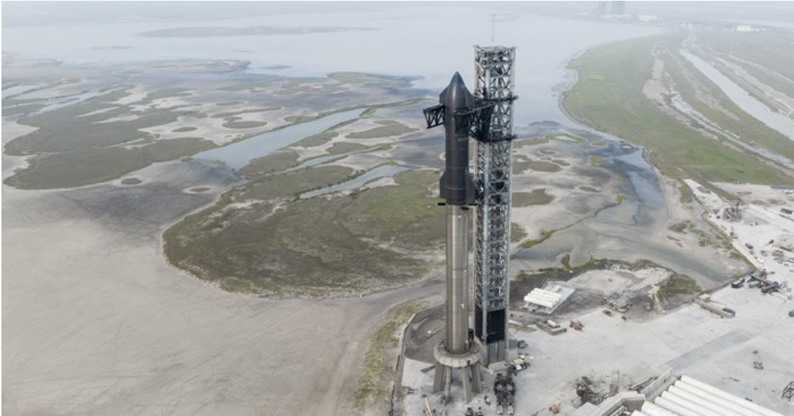
Starship mounted on the Super Heavy first stage booster ahead of its recent test launch. Source: SpaceX/Flickr
